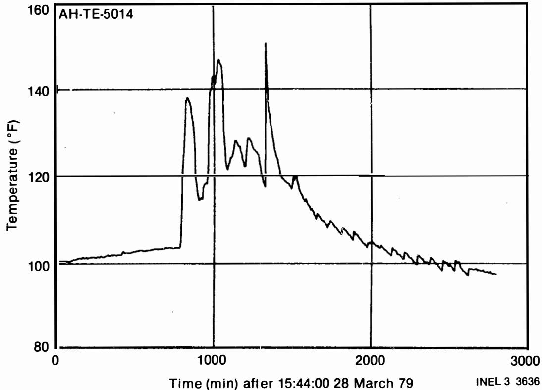
Figure A-6. Lower equipment hatch ambient air temp 305 (long term trend).
