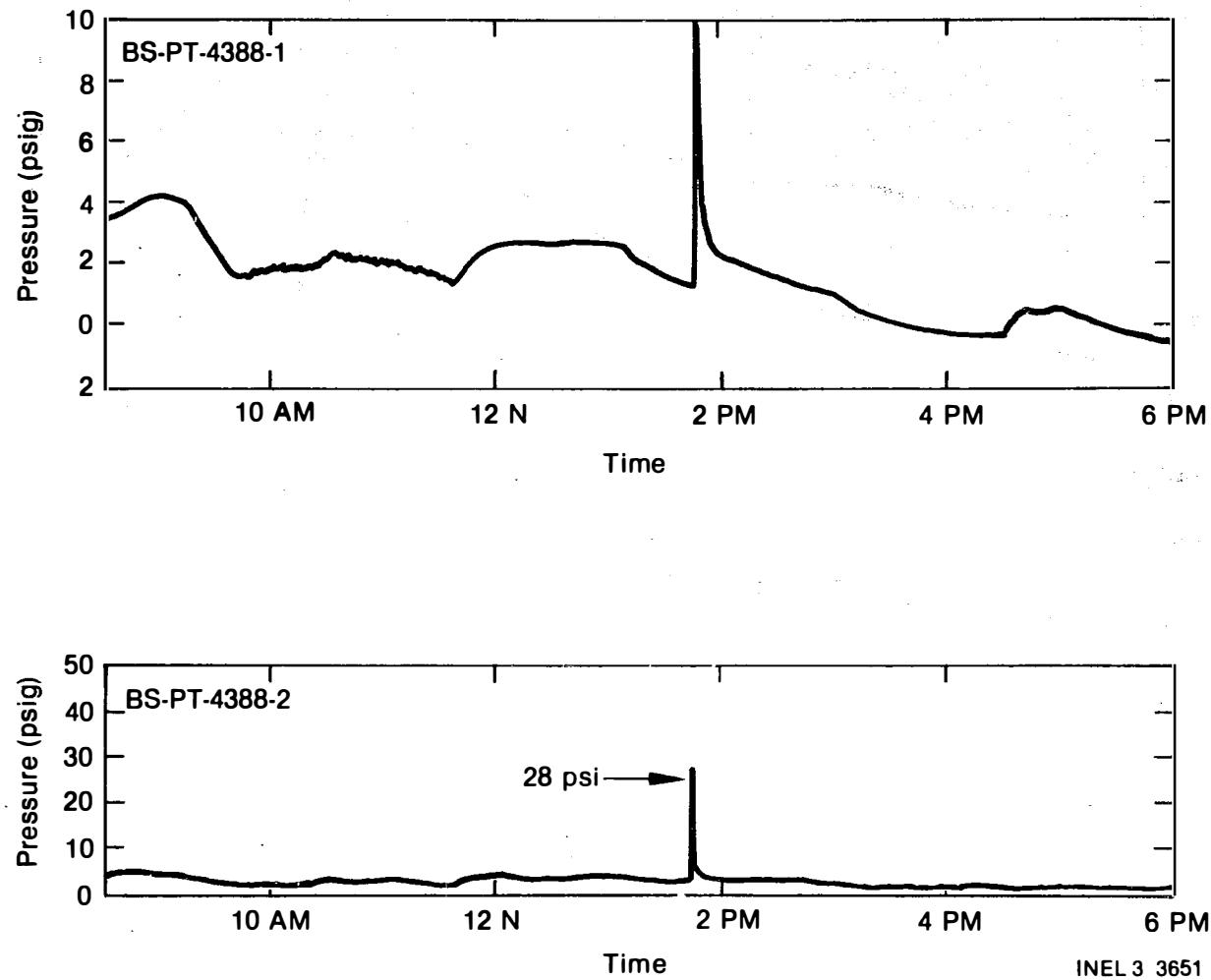
Figure C-1. Reactor Building pressure stripchart records (28 March 1979).
