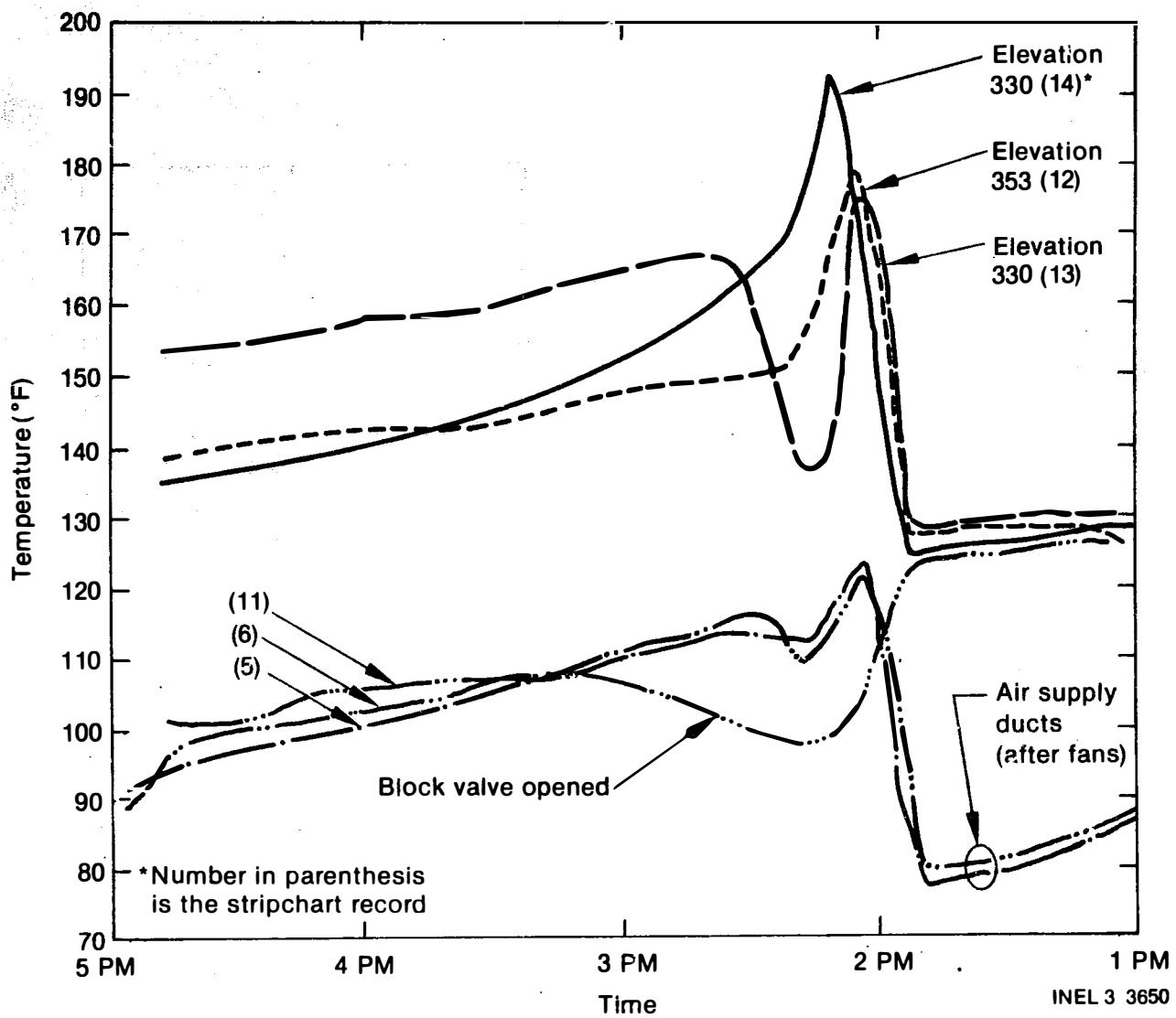
Figure C-2. Reactor Building resistance temperature detector readouts.
